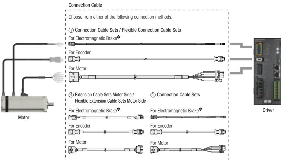
\*Required for motors with an electromagnetic brake.
