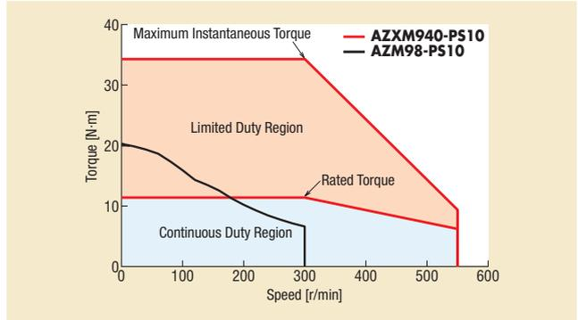
● This is a comparison of the speed – torque characteristics of the **AZX** Series and **AZ** Series.
