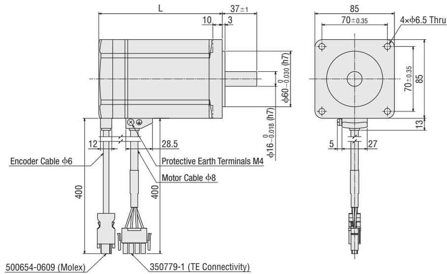
◇ Standard Type with an Electromagnetic Brake
