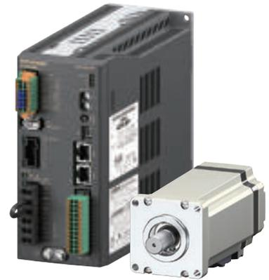
These servo motors are equipped with a battery-free absolute sensor. They are suitable for positioning applications with a large amount of travel, since they achieve high torque in the high speed range. The basic operations are the same as the **AZ** Series, making combined use in equipment easy.
