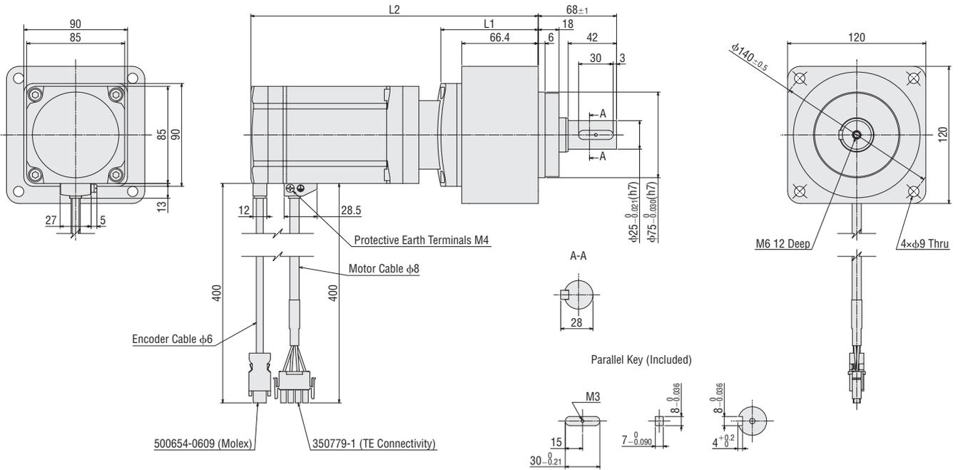
● A number indicating the gear ratio is specified where the box ■ is located in the product name.
